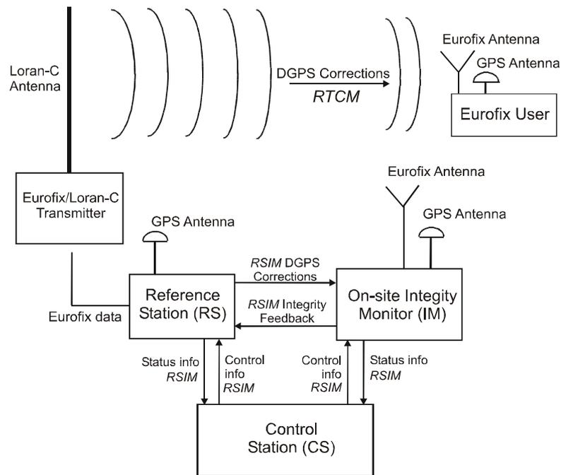
Figure 1. The building blocks of the Eurofix GNSS service, and the communication protocols that are used for each of the interfaces. RSIM is used internally within the reference station infrastructure, while the RTCM protocol is used for the broadcast to the user.
